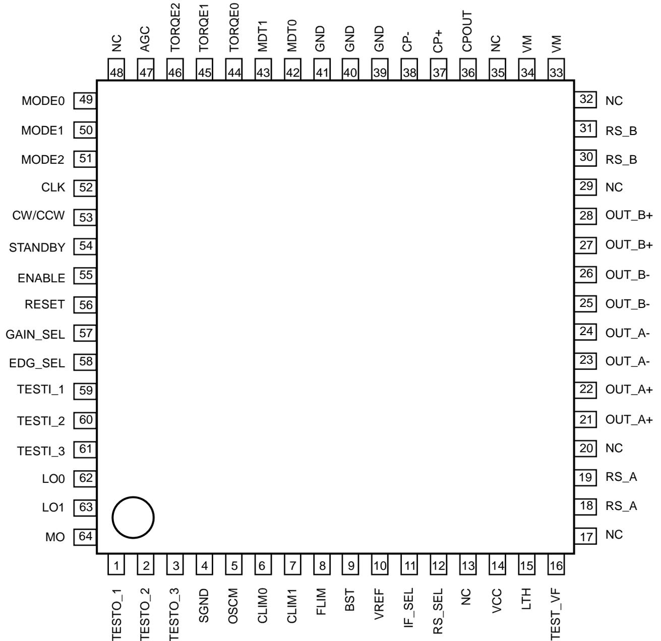
Note: Please solder the corner pads and the rear thermal pad of the QFN package, to the GND pattern of the PCB.
