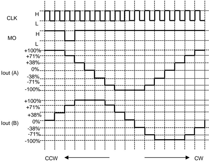
Note: MO signal is shown in the above timing chart when MO pin is connected with a pull-up resistor to VCC.
