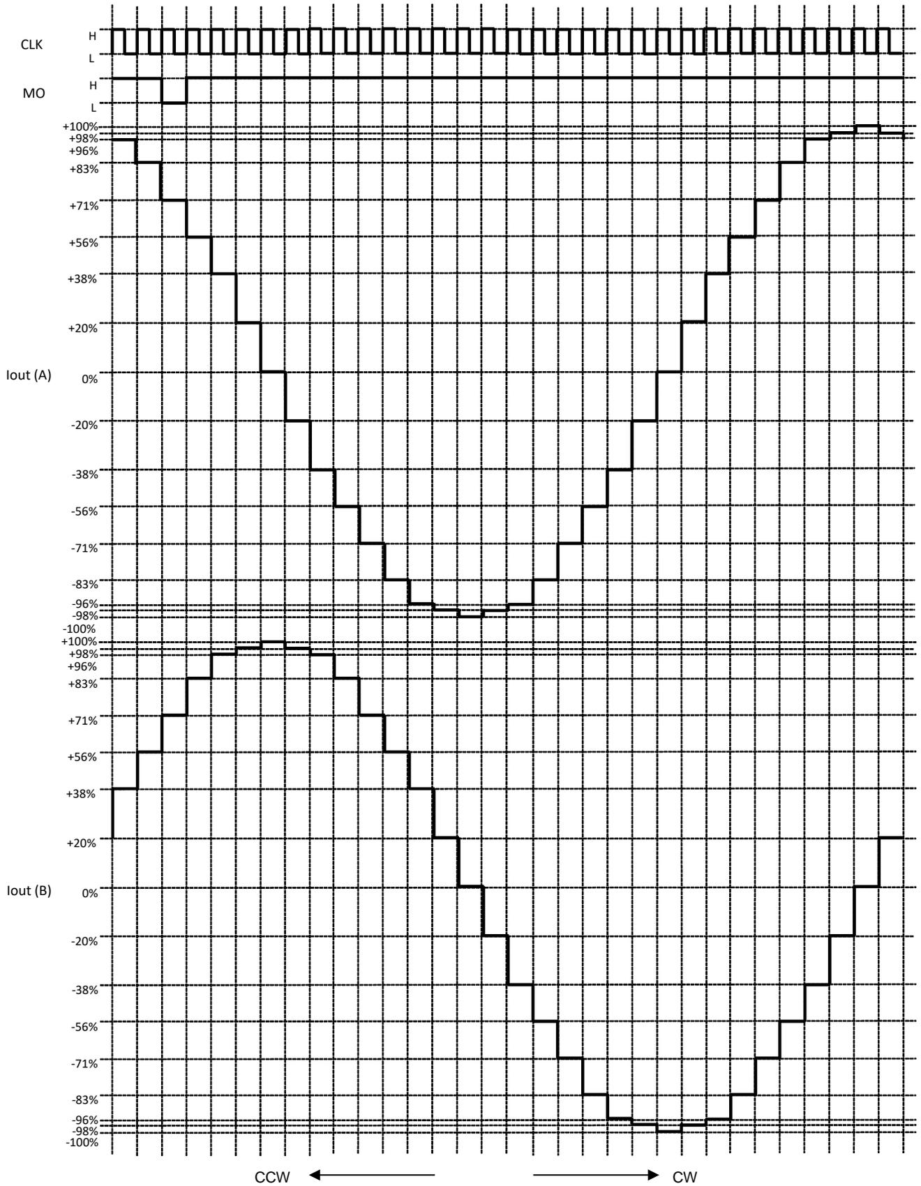
Note: MO signal is shown in the above timing chart when MO pin is connected with a pull-up resistor to VCC.
