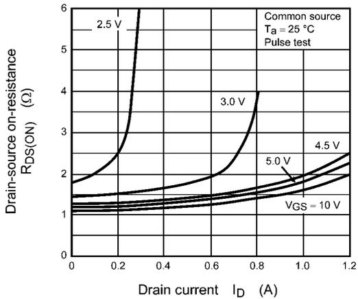
Fig. 7.3  $R_{DS(ON)} - I_D$
