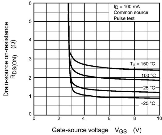
Fig. 7.4  $R_{DS(ON)} - V_{GS}$
