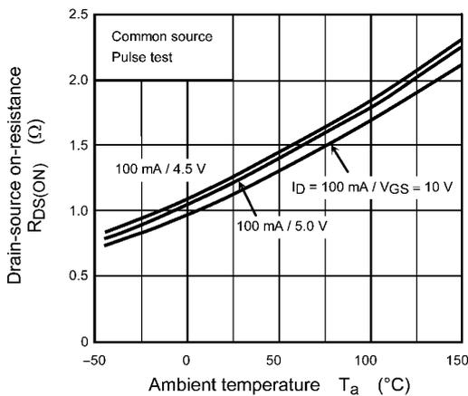
Fig. 7.5  $R_{DS(ON)} - T_a$
