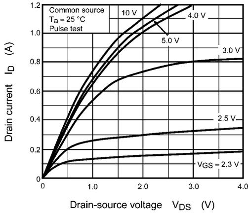
**Fig. 7.1  $I_D - V_{DS}$**
