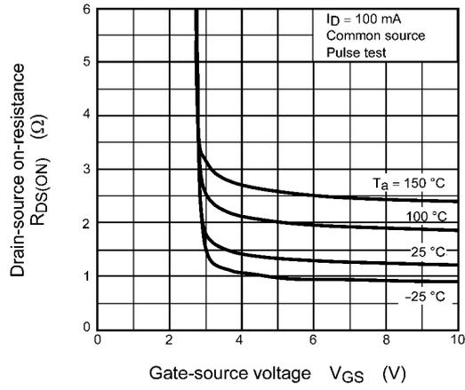
**Fig. 7.4  $R_{DS(ON)} - V_{GS}$**
