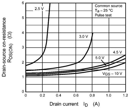
**Fig. 7.3  $R_{DS(ON)} - I_D$**
