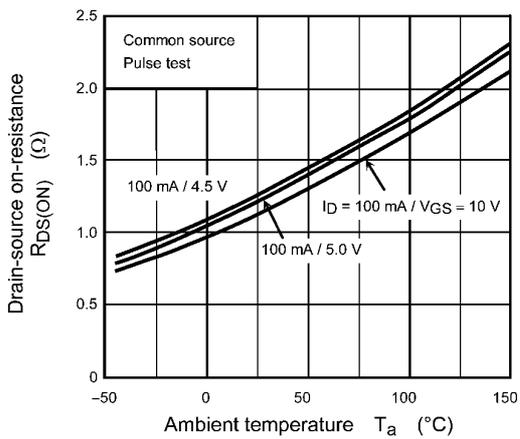
**Fig. 7.5  $R_{DS(ON)} - T_a$**
