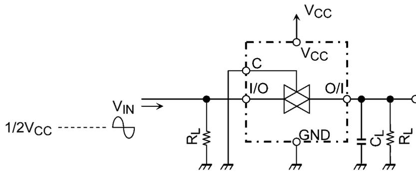
**Figure 4 Feedthrough**
