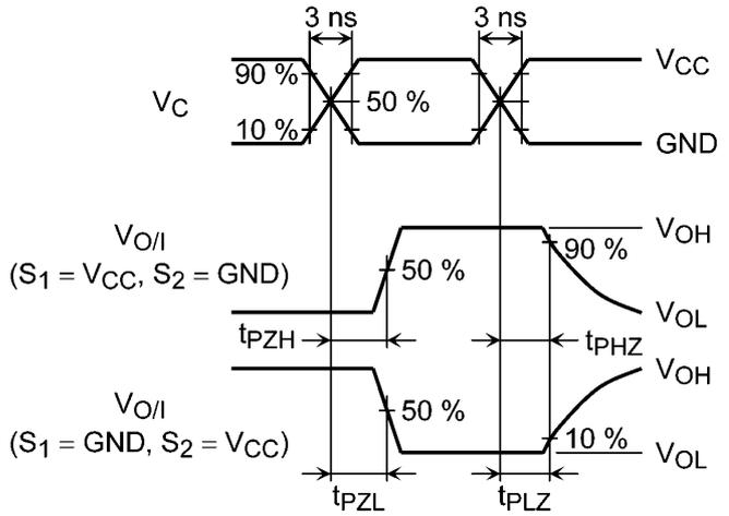
Figure 1  $t_{PZH}$ ,  $t_{PHZ}$ ,  $t_{PZL}$ ,  $t_{PLZ}$
