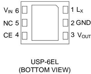
\* The dissipation pad for the USP-6EL package should be solder-plated in reference mount pattern and metal masking so as to enhance mounting strength and heat release. The mount pattern should be connected to GND pin (No.2).
