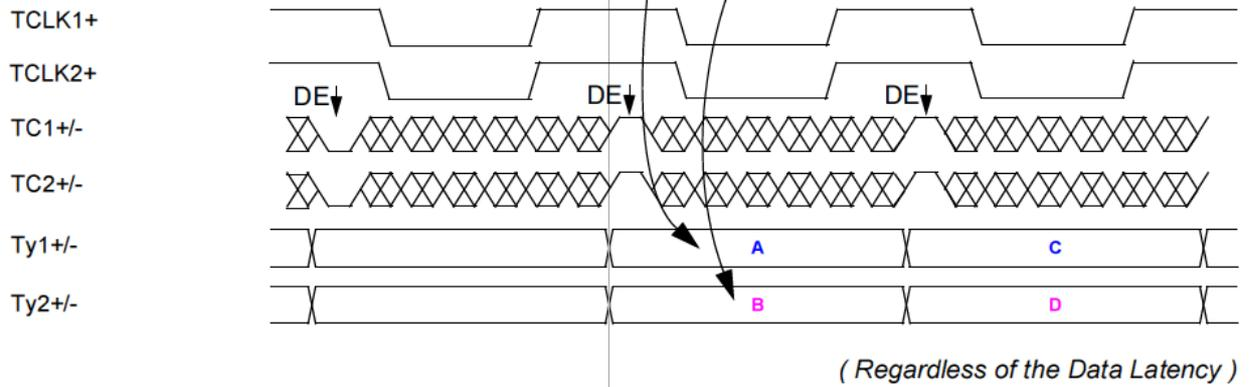
**Schematic diagram of DE transition**
