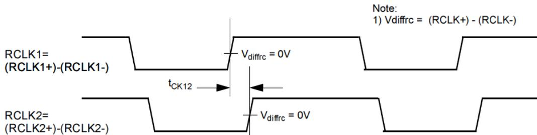
**Figure 11. Skew time between RCLK1 and RCLK2**
