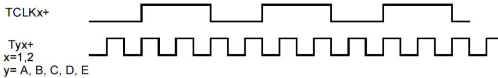
**Figure 5. Test Pattern (LVDS Output Full Toggle Pattern)**
