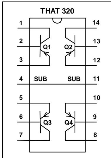
Figure 2. 320 Pinout
