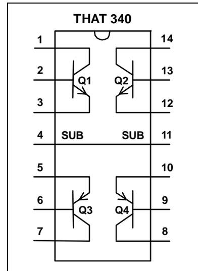
Figure 3. 340 Pinout
