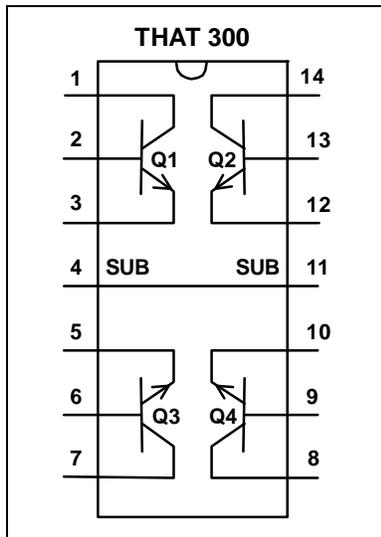
Figure 1. 300 Pinout
