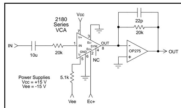
Figure 14. Positive control port using Pin 2 ( $E_{c+}$ )
