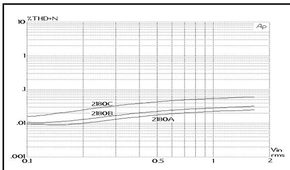
Figure 11. 1 kHz THD+Noise vs. Input Level, +15dB gain
