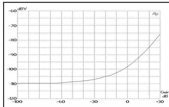
Figure 4. 2180-series Noise (20kHz NBW) vs. Gain
