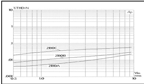
Figure 10. 1 kHz THD+Noise vs. Input Level, 0dB gain
