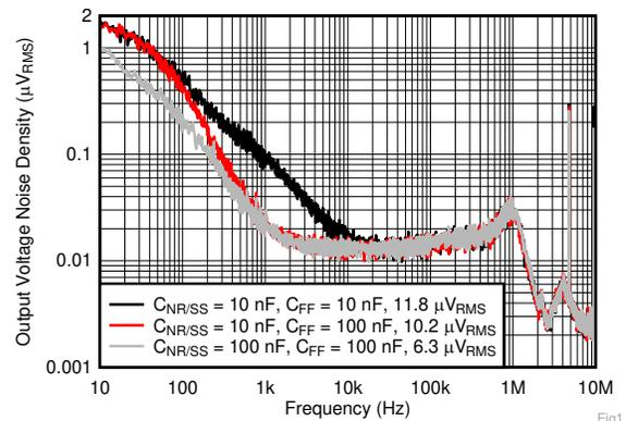
$I_{OUT} = 2\text{ A}$ ,  $C_{OUT} = 22\ \mu\text{F}$ ,  $C_{FF} = 10\text{ nF}$ ,
