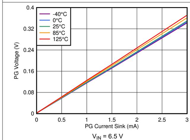
图 7-41. PG Voltage vs PG Current Sink
