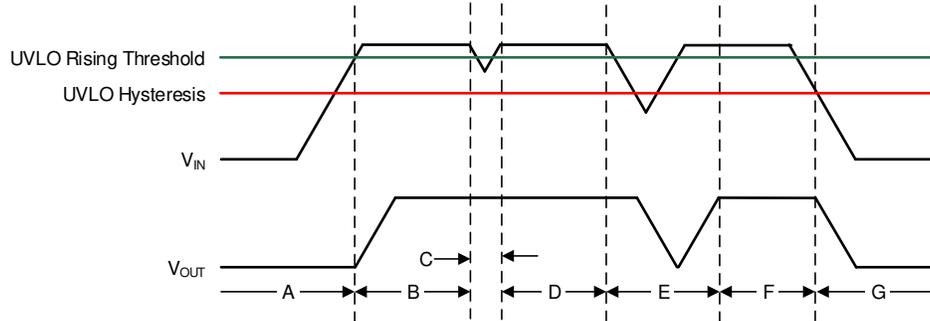
图 9-4. Typical UVLO Operation
