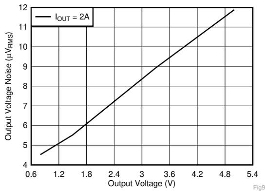
$V_{IN} = V_{OUT} + 0.3\text{ V}$  and  $V_{BIAS} = 5\text{ V}$  for  $V_{OUT} \leq 2.2\text{ V}$ ,
