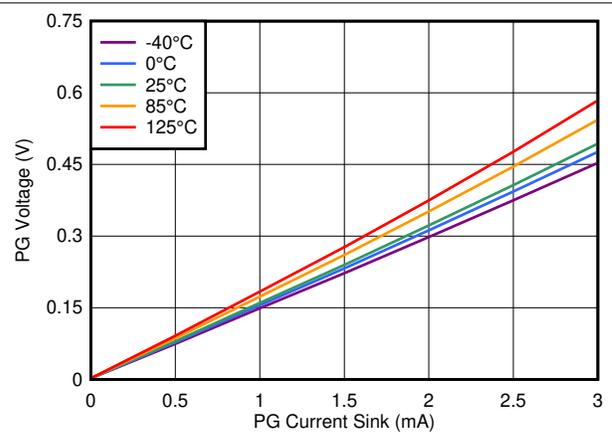
图 7-40. PG Voltage vs PG Current Sink
