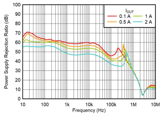
$V_{IN} = 5.5\text{ V}$ ,  $V_{OUT} = 5\text{ V}$ ,  $C_{OUT} = 47\ \mu\text{F} \parallel 10\ \mu\text{F} \parallel 10\ \mu\text{F}$ ,
