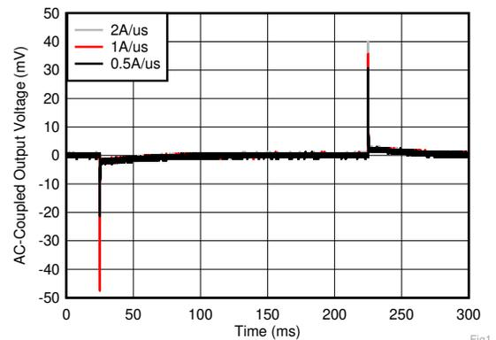
$V_{OUT} = 5\text{ V}$ ,  $I_{OUT,DC} = 100\text{ mA}$ ,  $I_{OUT} = 100\text{ mA}$  to  $2\text{ A}$ ,
