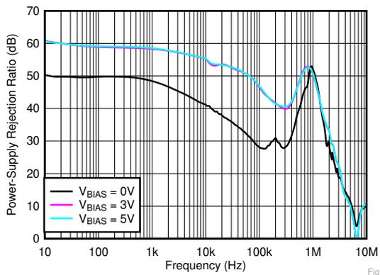
$V_{IN} = 1.4\text{ V}$ ,  $I_{OUT} = 1\text{ A}$ ,  $C_{OUT} = 22\ \mu\text{F}$ ,  $C_{NR/SS} = 10\text{ nF}$ ,
