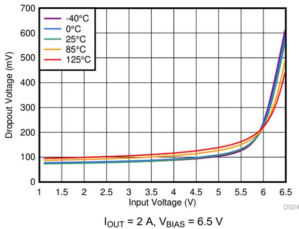
$I_{OUT} = 2\text{ A}$ ,  $V_{BIAS} = 6.5\text{ V}$
