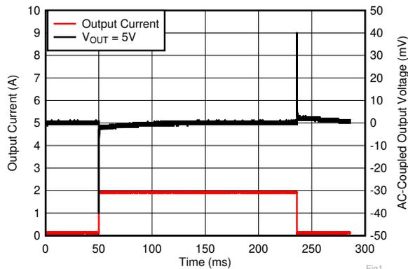
$I_{OUT,DC} = 100\text{ mA}$ ,  $C_{OUT} = 22\ \mu\text{F}$ ,  $C_{NR/SS} = C_{FF} = 10\text{ nF}$ ,
