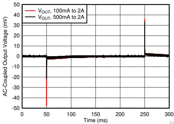
$V_{IN} = 5.3\text{ V}$ ,  $V_{BIAS} = 5\text{ V}$ ,  $C_{OUT} = 22\ \mu\text{F}$ ,  $C_{BIAS} = 10\ \mu\text{F}$ ,  $V_{OUT} = 5\text{ V}$ ,  $C_{NR/SS} = C_{FF} = 10\text{ nF}$ , slew rate =  $1\text{ A}/\mu\text{s}$
