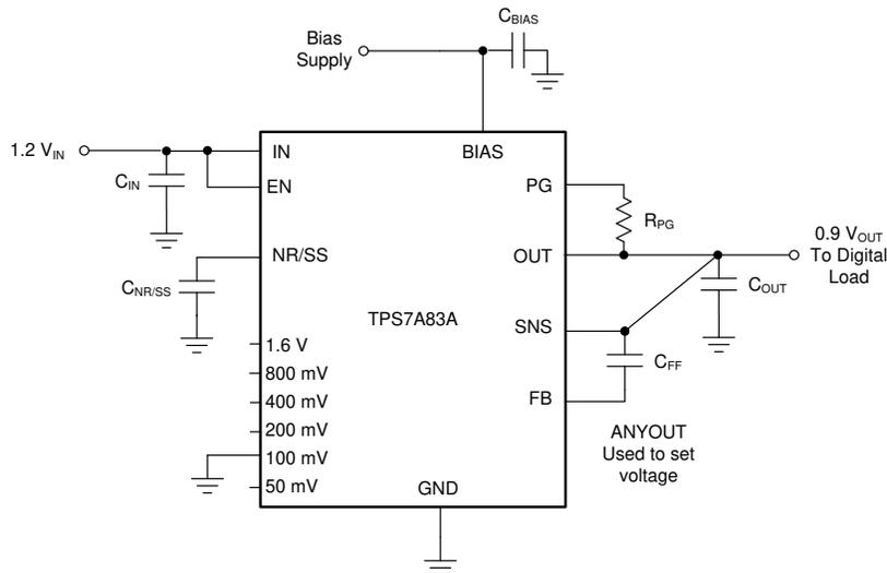
图 9-3. ANY-OUT Configuration Circuit (0.9-V Output With BIAS)
