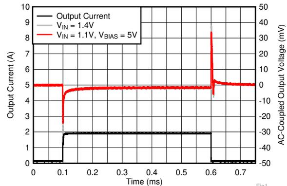
$I_{OUT,DC} = 100\text{ mA}$ , slew rate =  $1\text{ A}/\mu\text{s}$ ,  $C_{NR/SS} = 10\text{ nF}$ ,
