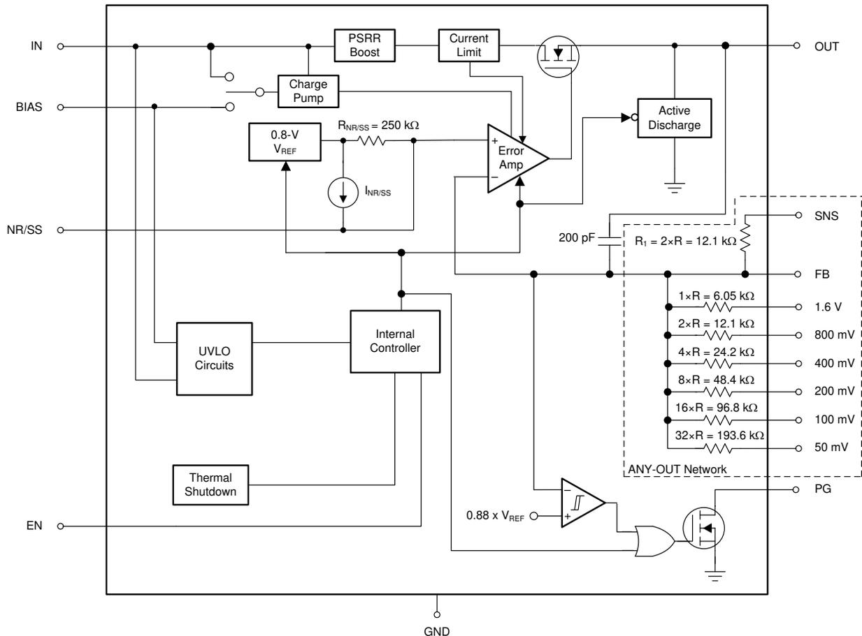
NOTE: For the ANY-OUT network, the ratios between the values are highly accurate as a result of matching, but the actual resistance can vary significantly from the numbers listed.
