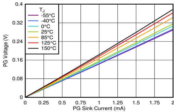
图 7-65. PG Voltage vs PG Current Sink
