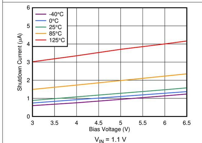
图 7-35. Shutdown Current vs Bias Voltage
