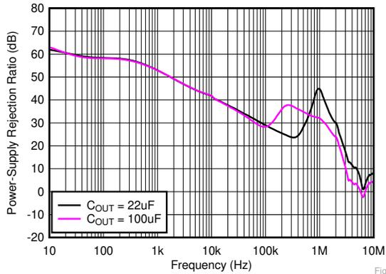
$V_{IN} = V_{OUT} + 0.3\text{ V}$ ,  $V_{OUT} = 1\text{ V}$ ,  $V_{BIAS} = 5\text{ V}$ ,  $I_{OUT} = 2\text{ A}$ ,
