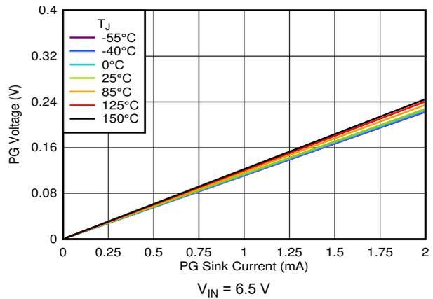
图 7-66. PG Voltage vs PG Current Sink
