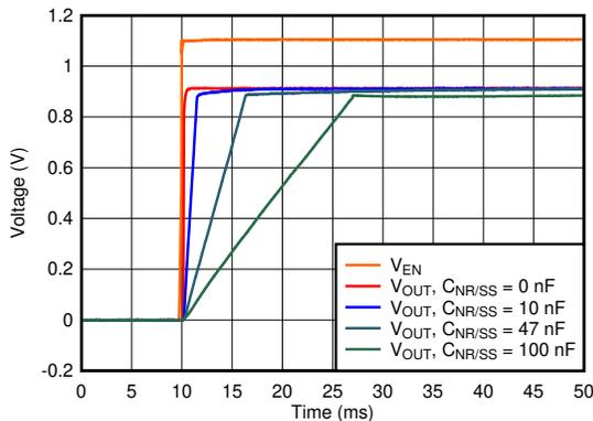
$V_{IN} = 1.2\text{ V}$ ,  $V_{OUT} = 0.9\text{ V}$ ,  $V_{BIAS} = 5\text{ V}$ ,  $I_{OUT} = 2\text{ A}$ ,
