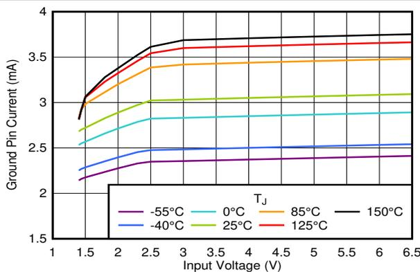
$V_{BIAS} = 0\text{ V}$ ,  $I_{OUT} = 5\text{ mA}$
