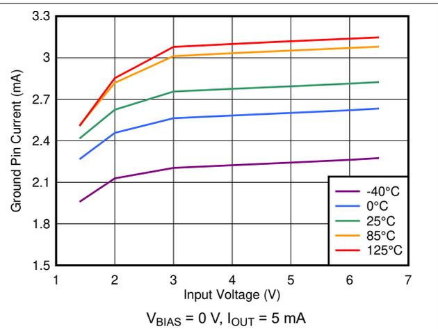
图 7-32. Ground Pin Current vs Input Voltage
