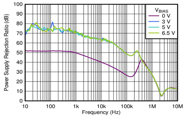
$V_{IN} = 1.4\text{ V}$ ,  $I_{OUT} = 1\text{ A}$ ,  $C_{OUT} = 22\ \mu\text{F}$ ,  $C_{NR/SS} = 10\text{ nF}$ ,
