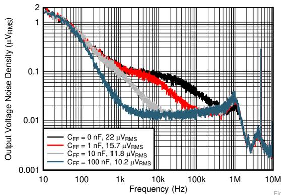
$V_{IN} = 5.3\text{ V}$ ,  $V_{OUT} = 5\text{ V}$ ,  $V_{BIAS} = 5\text{ V}$ ,  $I_{OUT} = 2\text{ A}$ ,  $C_{OUT} = 22\ \mu\text{F}$ ,
