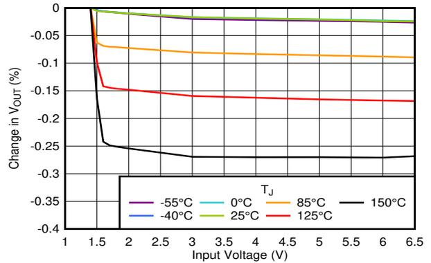
$V_{OUT} = 0.5\text{ V}$ ,  $I_{OUT} = 5\text{ mA}$
