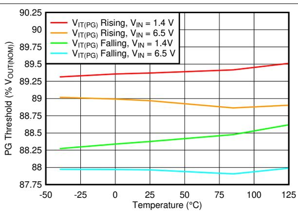
图 7-42. PG Threshold vs Temperature
