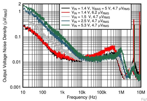
$I_{OUT} = 2\text{ A}$ ,  $C_{OUT} = 22\ \mu\text{F}$ ,  $C_{NR/SS} = 10\text{ nF}$ ,  $C_{FF} = 10\text{ nF}$ ,
