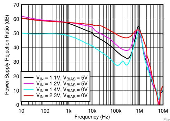
$I_{OUT} = 1\text{ A}$ ,  $C_{OUT} = 22\ \mu\text{F}$ ,  $C_{NR/SS} = 10\text{ nF}$ ,  $C_{FF} = 10\text{ nF}$
