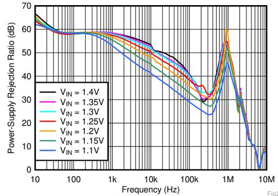
$I_{OUT} = 2\text{ A}$ ,  $V_{BIAS} = 5\text{ V}$ ,  $C_{OUT} = 22\ \mu\text{F}$ ,  $C_{NR/SS} = 10\text{ nF}$ ,
