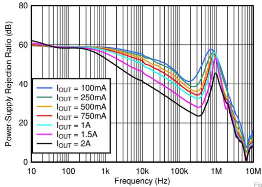
$V_{IN} = 1.1\text{ V}$ ,  $V_{BIAS} = 5\text{ V}$ ,  $C_{OUT} = 22\ \mu\text{F}$ ,  $C_{NR/SS} = 10\text{ nF}$ ,
