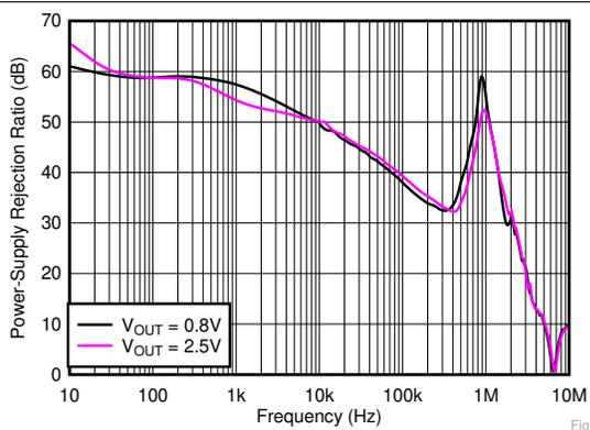
$V_{IN} = V_{OUT} + 0.3\text{ V}$ ,  $V_{BIAS} = 5\text{ V}$ ,  $I_{OUT} = 2\text{ A}$ ,  $C_{OUT} = 22\ \mu\text{F}$ ,
