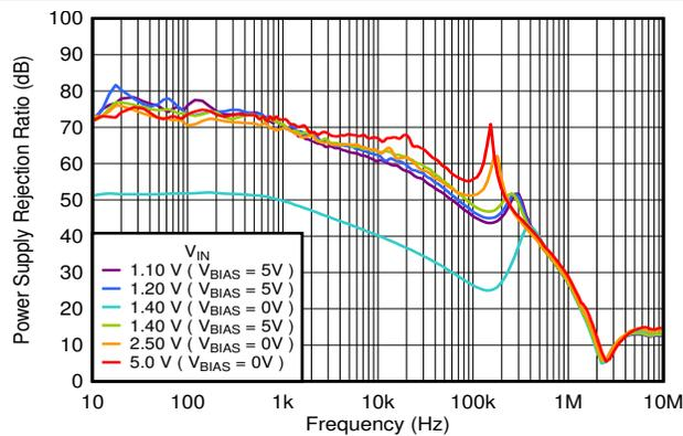
$I_{OUT} = 1\text{ A}$ ,  $C_{OUT} = 22\ \mu\text{F}$ ,  $C_{NR/SS} = 10\text{ nF}$ ,  $C_{FF} = 10\text{ nF}$
