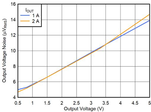
$V_{IN} = V_{OUT} + 0.3\text{ V}$  or  $V_{IN} = 1.1\text{ V}$  (whichever is greater) and
