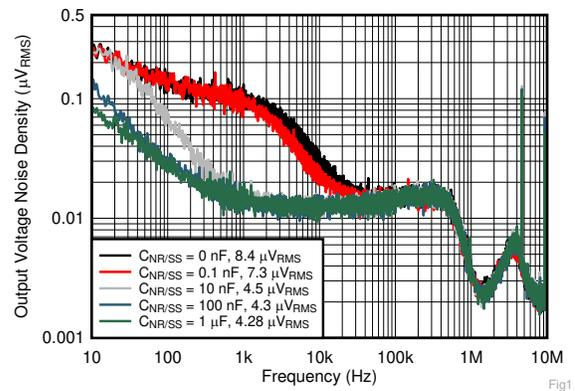
$V_{IN} = 1.1\text{ V}$ ,  $V_{OUT} = 0.8\text{ V}$ ,  $V_{BIAS} = 5\text{ V}$ ,  $I_{OUT} = 2\text{ A}$ ,
