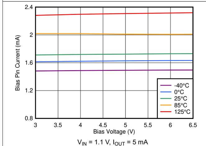
图 7-33. BIAS Pin Current vs Bias Voltage
