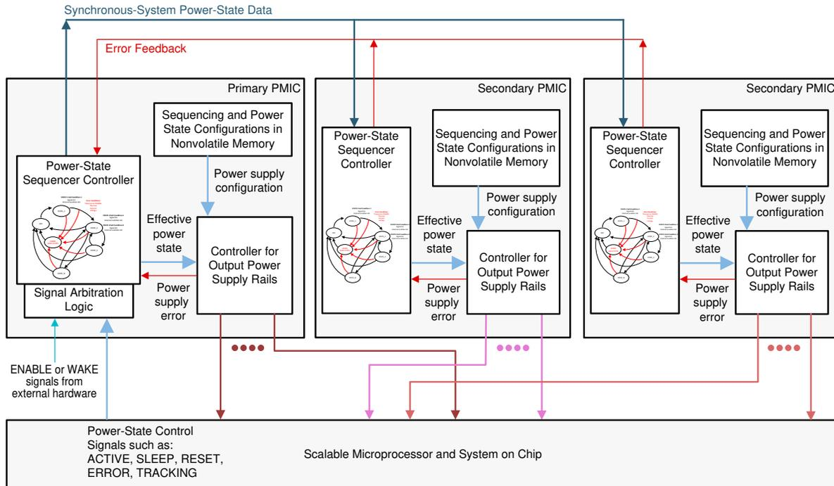
**图 8-46. Multi-PMIC Power State Synchronization Block Diagram**
