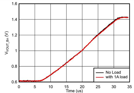
$V_{PVIN\_Bn} = 3.3\text{ V}$  Buck VSET = 0.6 V Slew Rate = 33.3 V/ms to 1.4 V
