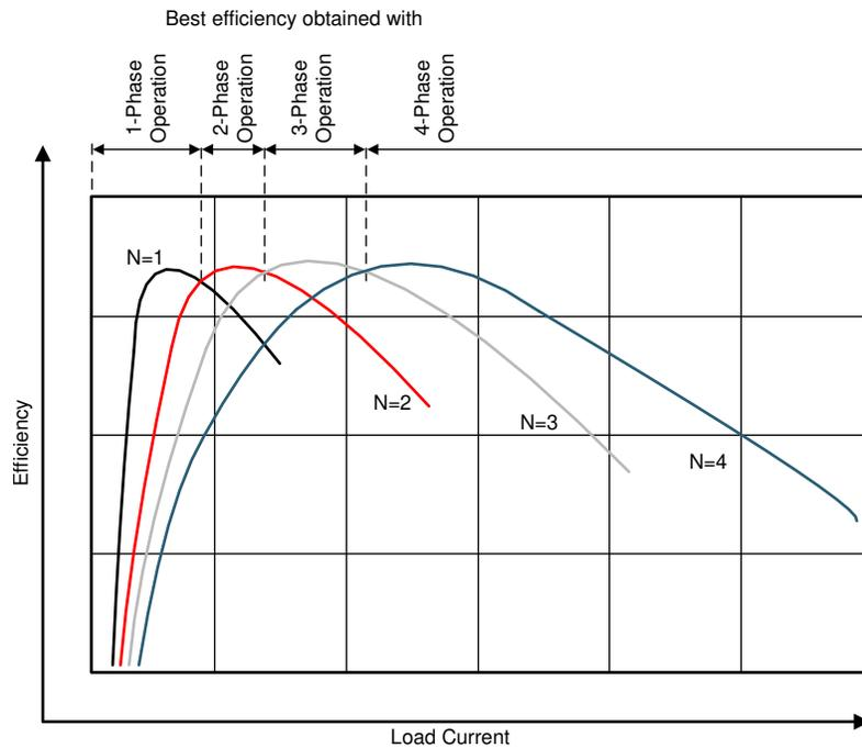
图 8-4. Multiphase BUCK Converter Efficiency vs Number of Phases (Converters in PWM Mode)<sup>2</sup>
