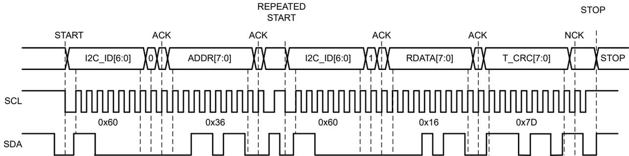
The I<sup>2</sup>C target device (i.e. the TPS6594-Q1) provides T\_CRC[7:0], which is calculated from the I2C\_ID, R/W, ADDR, I2C\_ID, R/W, and the RDATA bits (32 bits). See CRC Calculation for I2C and SPI Interface Protocols.
