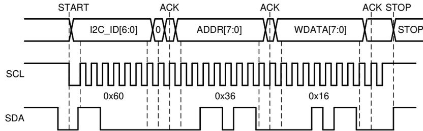
图 8-57. I<sup>2</sup>C Write Cycle without CRC
