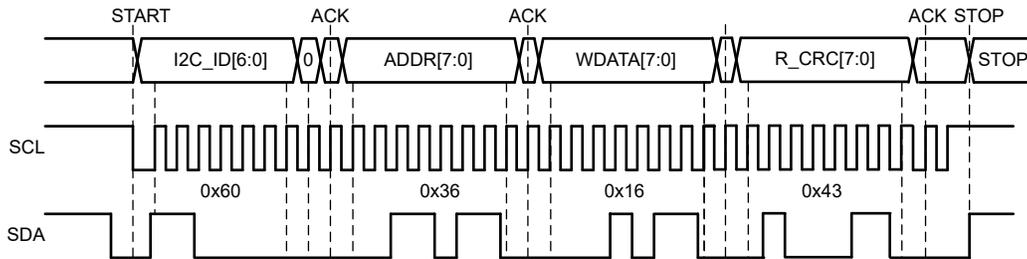
The I<sup>2</sup>C controller device (i.e. the MCU) provides R\_CRC[7:0], which is calculated from the I2C\_ID, R/W, ADDR, and the WDATA bits (24 bits). See CRC Calculation for I2C and SPI Interface Protocols.
