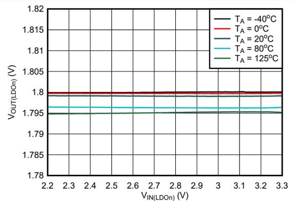
$V_{OUT(LDO_n)} = 1.8\text{ V}$   $I_{OUT(LDO_n)} = 50\text{ mA}$
