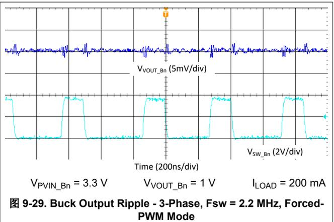
图 9-29. Buck Output Ripple - 3-Phase, Fsw = 2.2 MHz, Forced-PWM Mode
