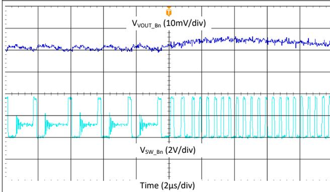
$V_{PVIN\_Bn} = 3.3\text{ V}$      $V_{VOUT\_Bn} = 1\text{ V}$      $I_{LOAD} = 200\text{ mA}$
