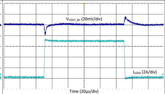
$I_{LOAD} = 0.1\text{ A} \rightarrow 7\text{ A} \rightarrow 0.1\text{ A}$ ,  $T_R = T_F = 1\ \mu\text{s}$
