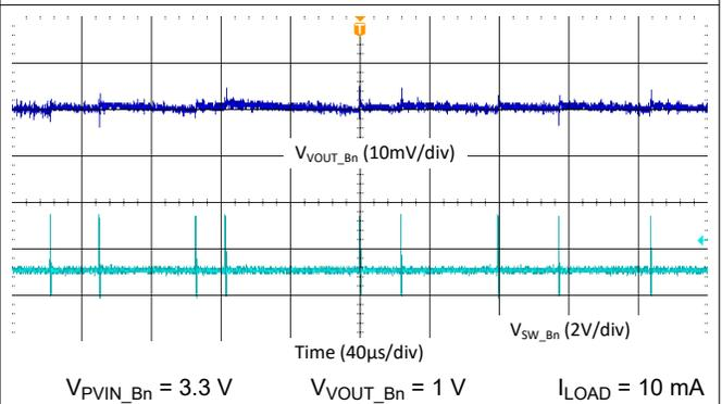
图 9-31. Buck Output Ripple - 4-Phase, Auto Mode
