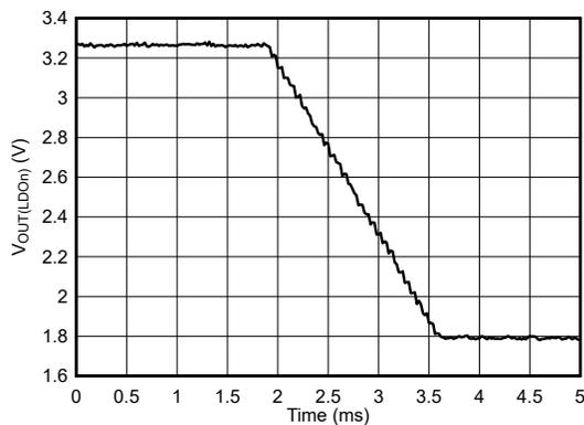
$V_{IN(LDO_n)} = 3.3\text{ V}$   $I_{OUT(LDO_n)} = 50\text{ mA}$
