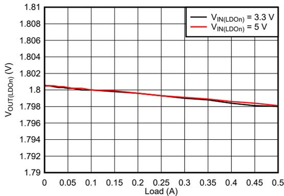
$V_{IN(LDO_n)} = 3.3\text{ V}$   $V_{OUT(LDO_n)} = 1.8\text{ V}$
