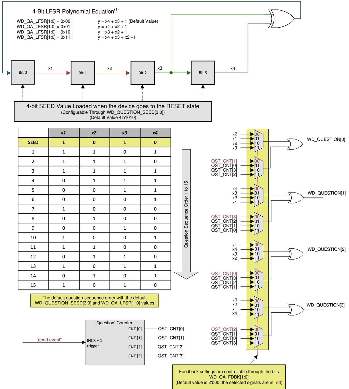
(1) If the current value for bits (x1, x2, x3, x4) is 4'b0000, the next value for these bits (x1, x2, x3, x4) is 4'b0001, and all further question generation begins from this value.
