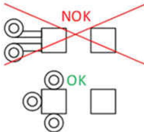
**图 11-1. Ground connection of capacitor at VOUT\_LDOVINT pin**
