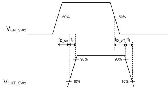
**Figure 1. Power Switches Test Circuit and Voltage Waveforms**
