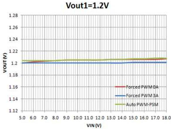
Figure 10. Line Regulation: Buck1 @ 1.2V, 1% Resistor Feedback
