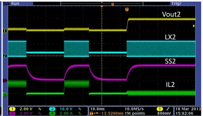
Figure 35. Hiccup Recover, Buck2=1.8V
