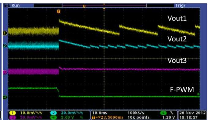
Figure 27. PSM/PWM Transition (Pin 25 Pulled Low)
