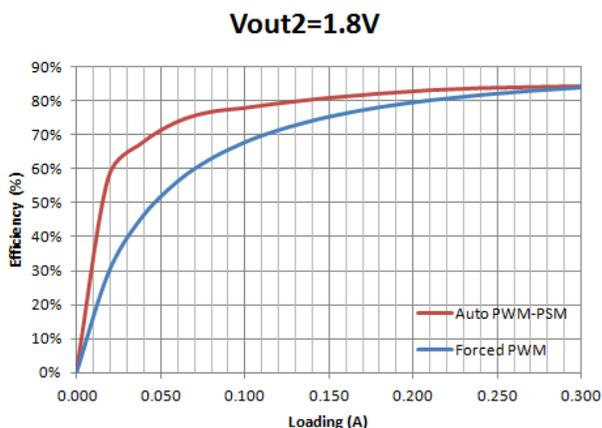
Figure 6. Buck2 1.8V Efficiency, Forced PWM and PSM
