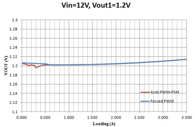
Figure 13. Load Regulation: Buck1 @ 1.2V, 1% Resistor Feedback
