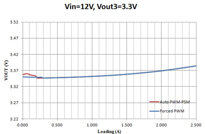
Figure 15. Load Regulation: Buck3 @ 3.3V, 1% Resistor Feedback
