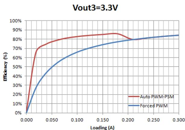
Figure 8. Buck3 3.3V Efficiency, Forced PWM and PSM
