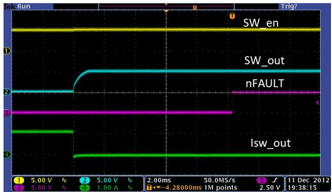
Figure 40. USB Switch Current Limit Recovery
