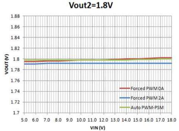
Figure 11. Line Regulation: Buck2 @ 1.8V, 1% Resistor Feedback
