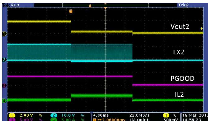
Figure 32. Over Current Protection and PGOOD Buck2=1.8V
