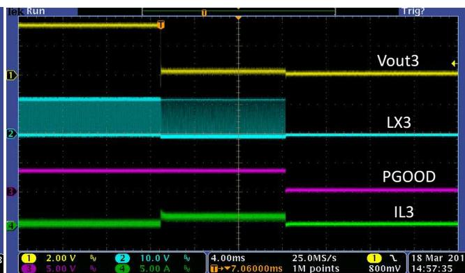
Figure 33. Over Current Protection and PGOOD Buck3=3.3V
