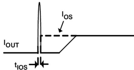
**Figure 2. Response Time to Short Circuit Waveform**
