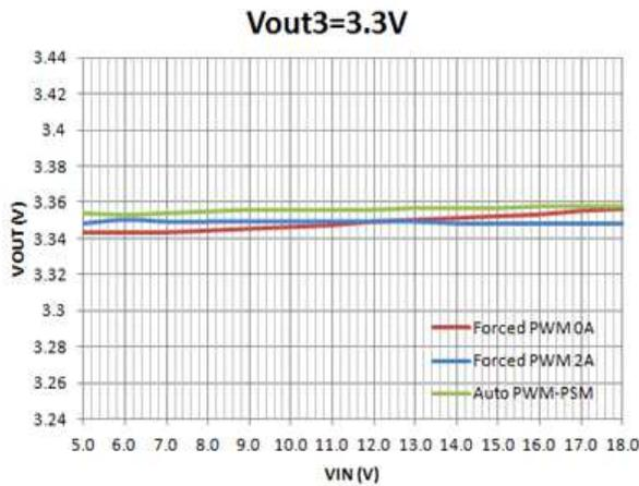
Figure 12. Line Regulation: Buck3 @ 3.3V, 1% Resistor Feedback
