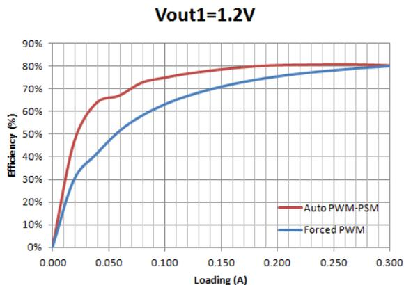
Figure 4. Buck1 1.2V Efficiency, Forced PWM and PSM
