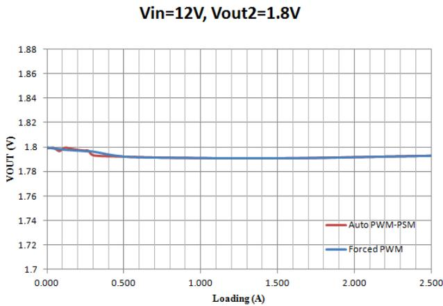
Figure 14. Load Regulation: Buck2 @ 1.8V, 1% Resistor Feedback
