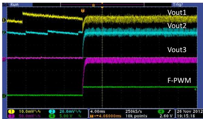
Figure 26. PSM/PWM Transition (Pin 25 Pulled High)
