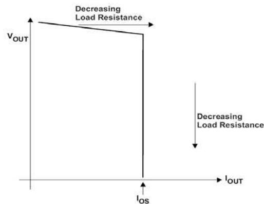
**Figure 3. Output Voltage vs Current Limit Threshold**
