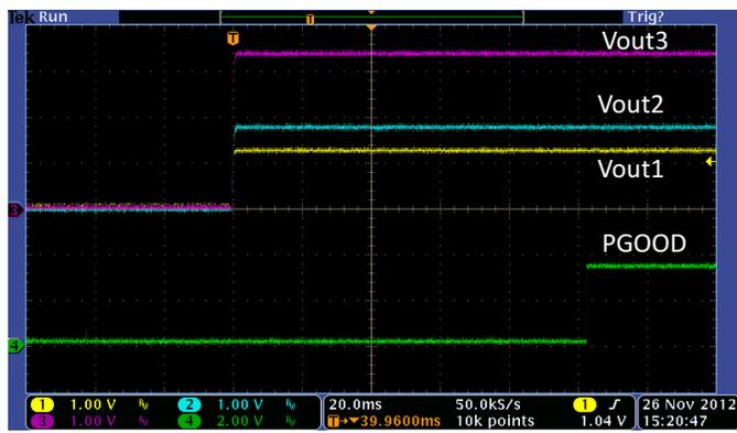
Figure 18. Power-Up All Converters and PGOOD, No Load
