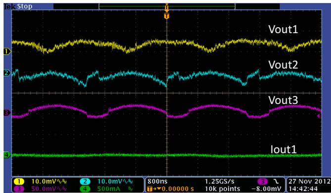
Figure 20. Ripple, Buck1 = 0A, Buck2 = 0A, Buck3 = 0A
