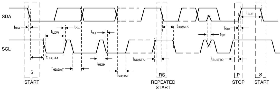
Figure 7-6. I<sup>2</sup>C-Compatible Timing
