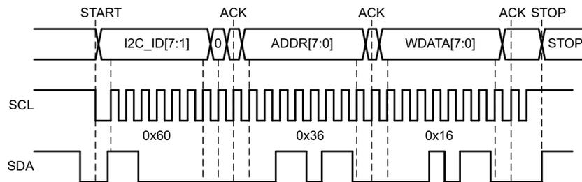
Figure 7-8. I<sup>2</sup>C Write Cycle without CRC
