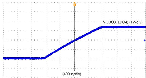
$V_{IN} = 5.0\text{ V}$        $V_{OUT} = 3.3\text{ V}$        $T_A = 25\text{ }^\circ\text{C}$
