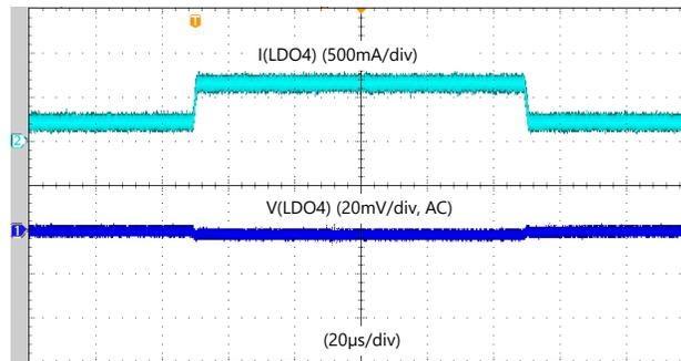
$V_{IN} = 3.3\text{ V}$        $V_{OUT} = 1.8\text{ V}$
