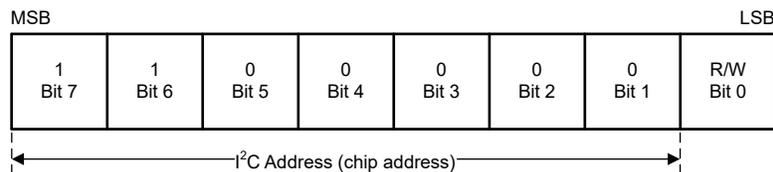
Figure 7-7. Example Device Address
