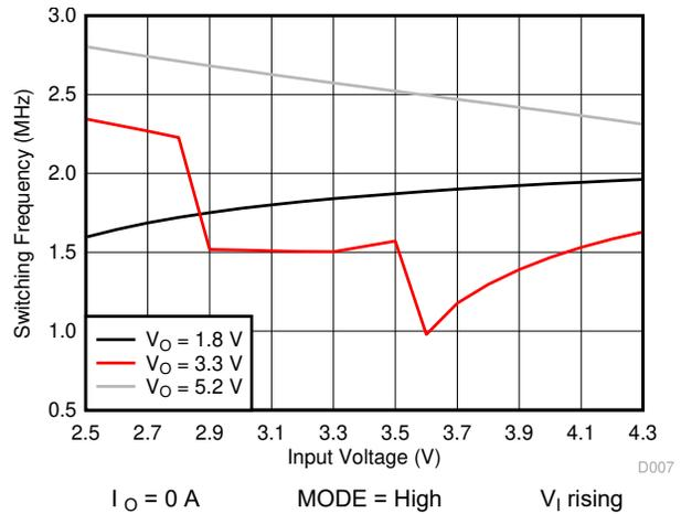
图 10-3. Typical Inductor Switching Frequency versus Input Voltage
