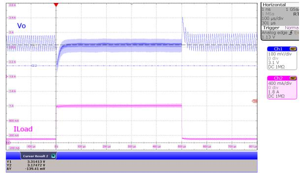
$V_I = 2.5 \text{ V}$ ,  $V_O = 3.3 \text{ V}$        $I_O$  from 100 mA to
