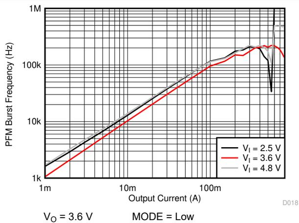
图 10-4. Typical Inductor Burst Frequency versus Output Current
