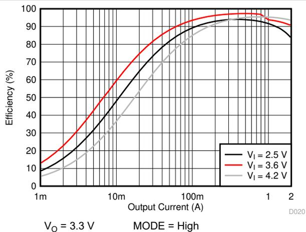
图 10-6. Efficiency versus Output Current (PWM Only)
