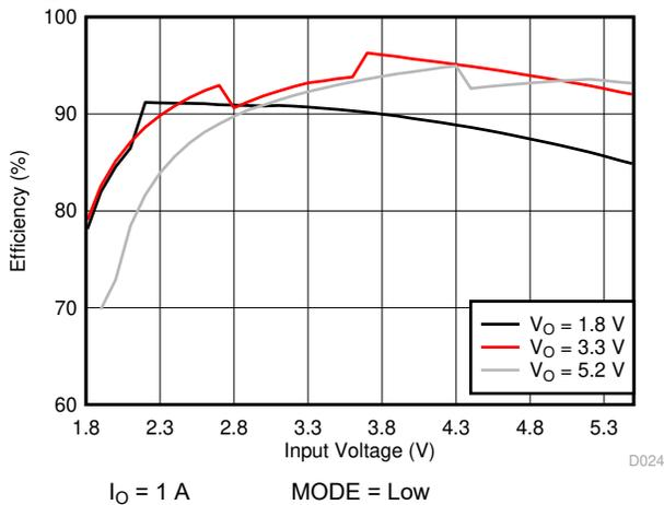
图 10-10. Efficiency versus Input Voltage (PWM Only)
