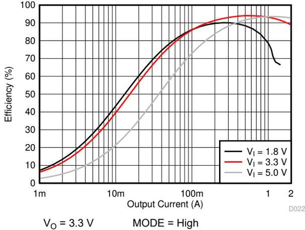
图 10-8. Efficiency versus Input Voltage (PWM Only)
