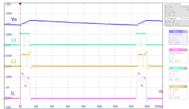
图 10-16. Switching Waveforms, PFM Buck-Boost Operation
