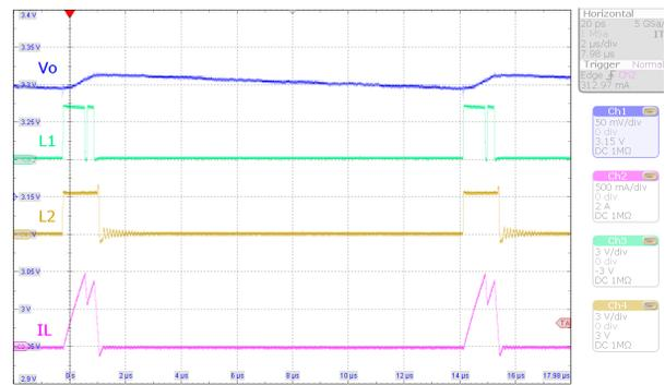
图 10-17. Switching Waveforms, PFM Buck Operation
