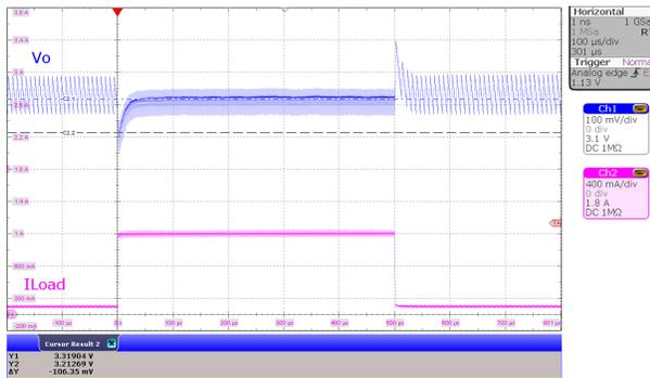
$V_I = 3.3 \text{ V}$ ,  $V_O = 3.3 \text{ V}$        $I_O$  from 100 mA
