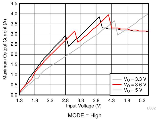
图 10-2. Typical Output Current Capability versus Input Voltage
