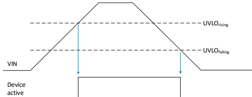
**图 9-3. Rising and Falling Undervoltage Lockout Behavior**
