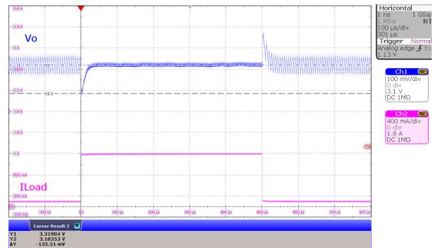
$V_I = 5 \text{ V}$ ,  $V_O = 3.3 \text{ V}$        $I_O$  from 100 mA
