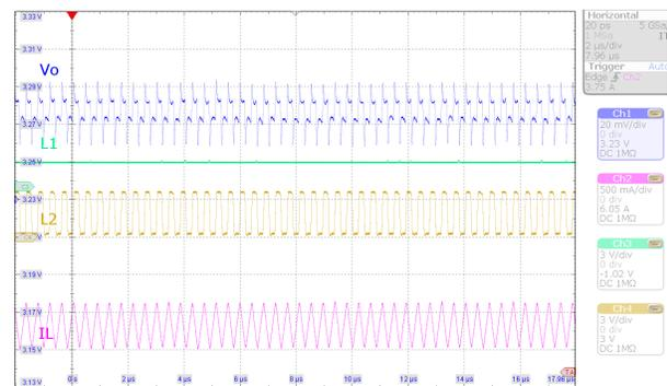
图 10-18. Switching Waveforms, PWM Boost Operation
