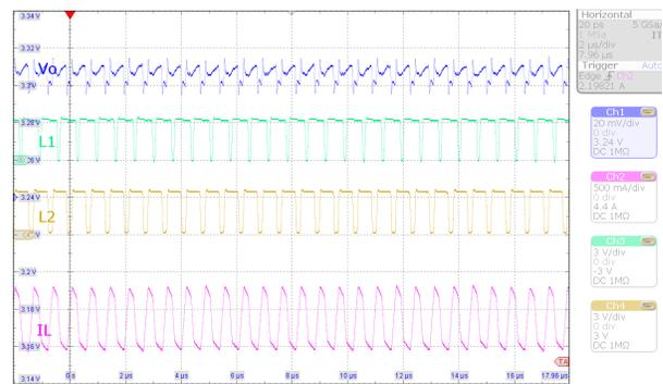
图 10-19. Switching Waveforms, PWM Buck-Boost Operation
