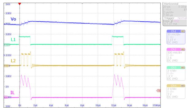
图 10-15. Switching Waveforms, PFM Boost Operation
