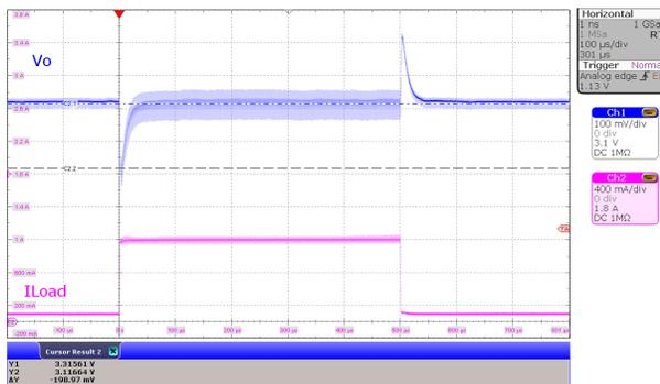
$V_I = 2.5 \text{ V}$ ,  $V_O = 3.3 \text{ V}$        $I_O$  from 100 mA
