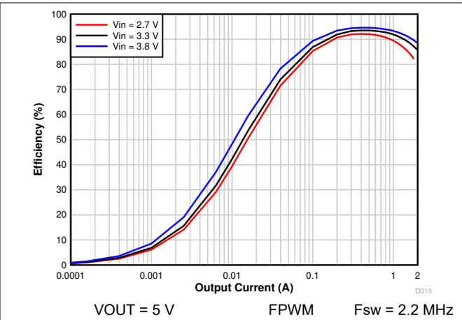
图 7-2. 5 V<sub>OUT</sub> Efficiency vs Output Current
