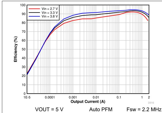
图 7-1. 5 V<sub>OUT</sub> Efficiency vs Output Current
