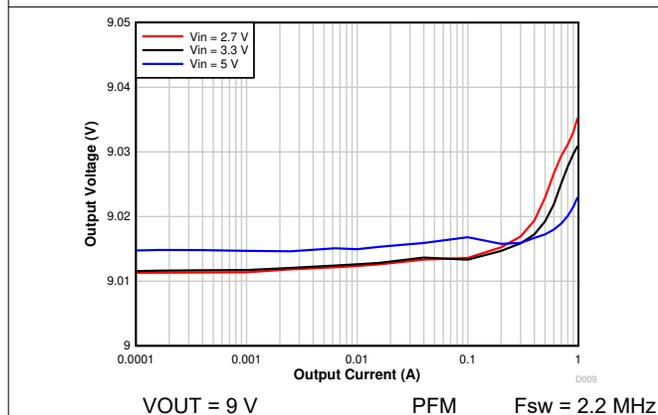
图 7-5. 9 V<sub>OUT</sub> Regulation vs Output Current
