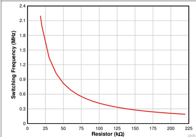
图 7-11. Switching Frequency vs Setting Resistance
