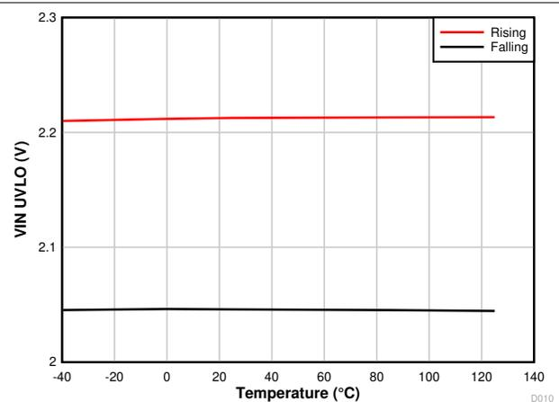
图 7-12.  $V_{IN}$  UVLO Threshold Voltage vs Temperature
