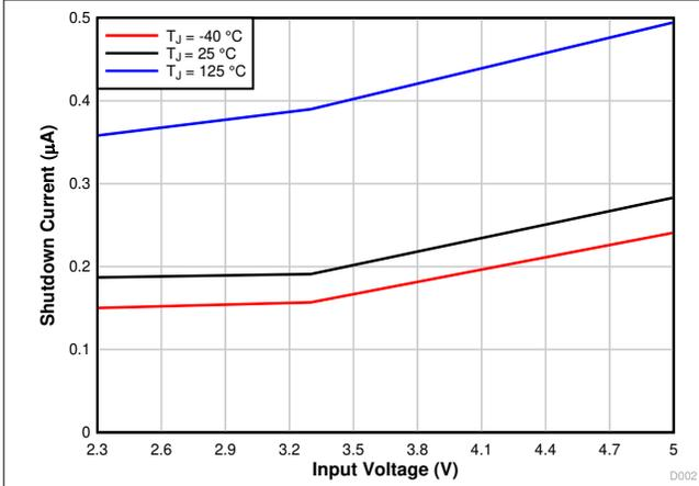
图 7-7. Shutdown Current vs Input Voltage
