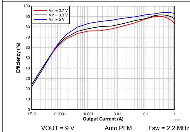
图 7-3. 9 V<sub>OUT</sub> Efficiency vs Output Current
