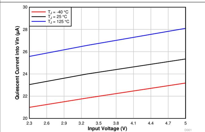
图 7-6. Quiescent Current into  $V_{IN}$  vs Input Voltage
