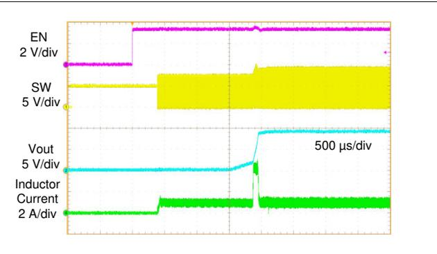
图 9-6. Start-up from EN Waveform  $V_{IN} = 5\text{ V}$ ,  $V_{OUT} = 9\text{ V}$ ,  $I_{OUT} = 500\text{ mA}$ , FPWM
