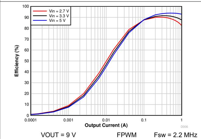
图 7-4. 9 V<sub>OUT</sub> Efficiency vs Output Current
