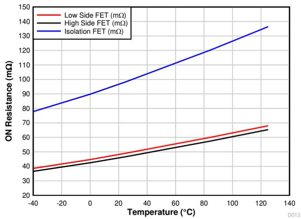
图 7-15. R<sub>DS(on)</sub> vs Temperature
