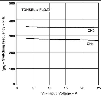
Figure 7. Switching Frequency (MED) vs Input Voltage
