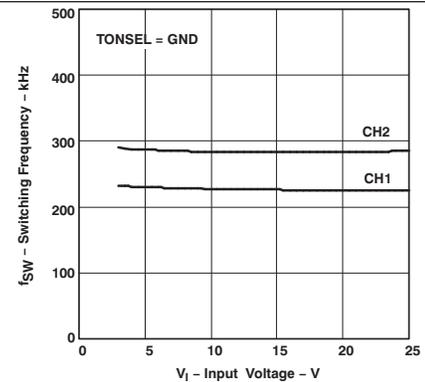
Figure 6. Switching Frequency (Slow) vs Input Voltage <sup>(1)</sup>
