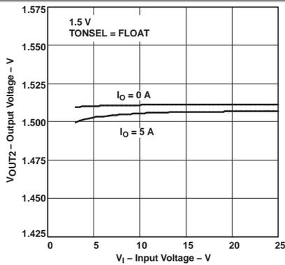
Figure 15. 1.5-V Output Voltage vs Input Voltage
