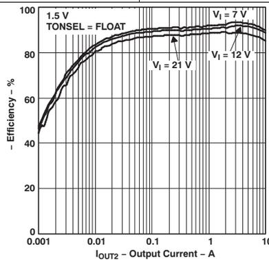
Figure 17. 1.5-V Efficiency vs Output Current <sup>(1)</sup>
