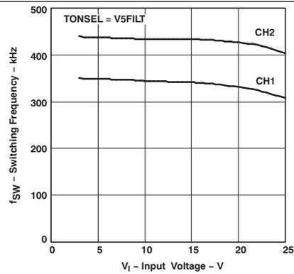
Figure 8. Switching Frequency (Fast) vs Input Voltage
