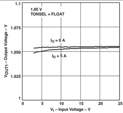
Figure 14. 1.05-V Output Voltage vs Input Voltage
