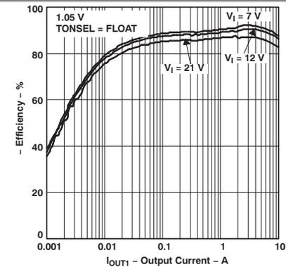
Figure 16. 1.05-V Efficiency vs Output Current
