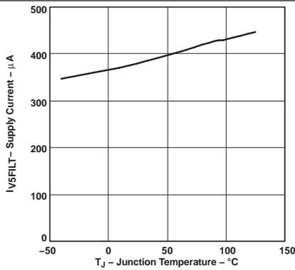
Figure 1. V5FILT Supply Current vs Junction Temperature
