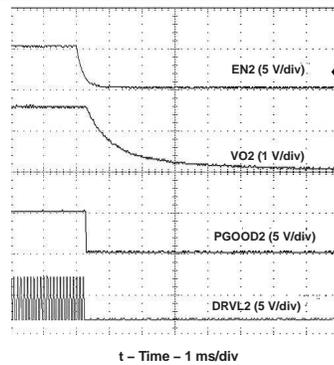
Figure 25. 1.5-V Discharge Waveforms
