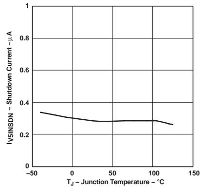
Figure 3. V5IN Shutdown Current vs Junction Temperature
