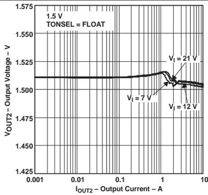
Figure 13. 1.5-V Output Voltage vs Output Current <sup>(1)</sup>
