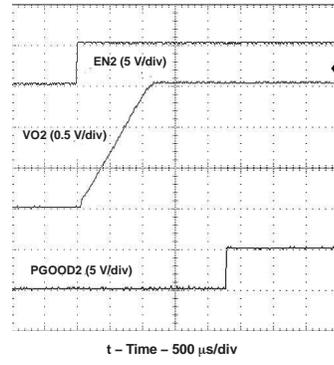
Figure 23. 1.5-V Start-Up Waveforms <sup>(1)</sup>
