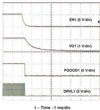
Figure 24. 1.05-V Discharge Waveforms
