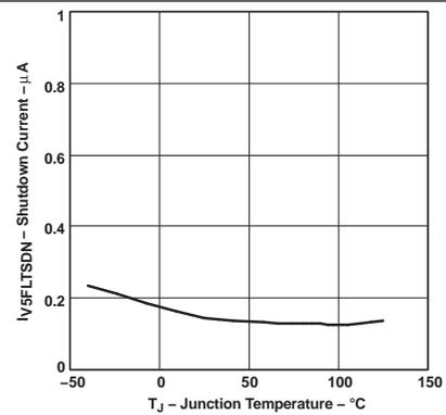
Figure 2. V5FILT Shutdown Current vs Junction Temperature
