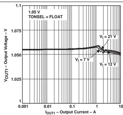
Figure 12. 1.05-V Output Voltage vs Output Current
