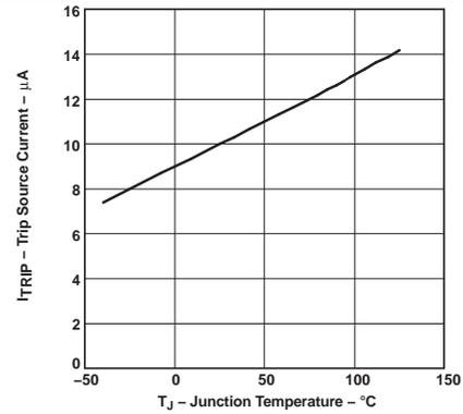
Figure 4. Trip Source Current vs Junction Temperature
