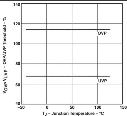
Figure 5. OVP/UVP Threshold vs Junction Temperature
