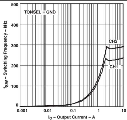
Figure 9. Switching Frequency (Slow) vs Output Voltage <sup>(1)</sup>
