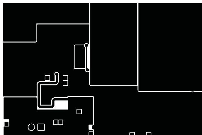
Figure 43. TPS40200EVM-001 Bottom Copper (X-Ray View From Top)
