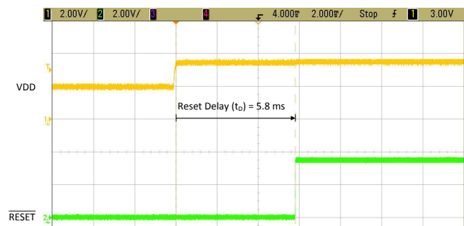
图 54. TPS3840EVM \overline{\text{RESET}} Time Delay ( t_D ) with 0.01- \mu F Capacitor
