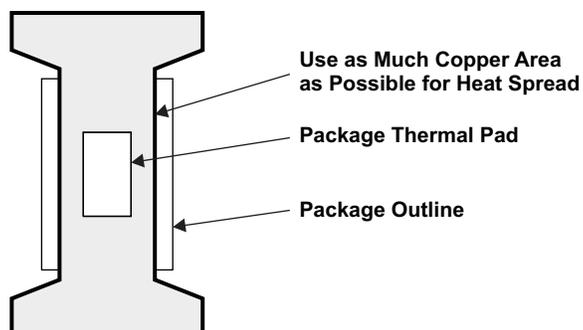
**Figure 6. Layout Recommendations for a Single-Layer PCB**
