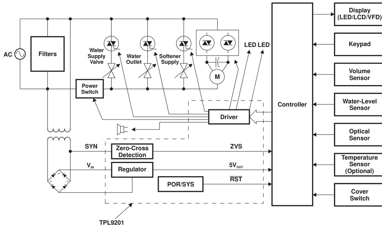
**Figure 3. Washing-Machine Application**
