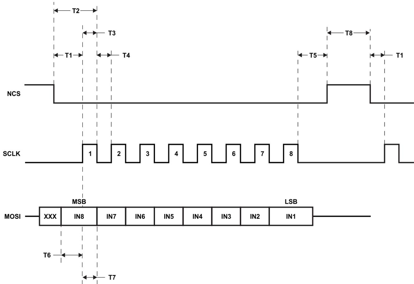
**Figure 1. Serial Communications**
