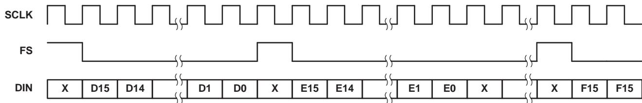
Difference between DSP mode (MODE = N.C. or 0) and  $\mu$ C (MODE = 1) mode:
