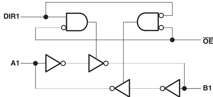
Figure 4. Logic Diagram (Positive Logic)
