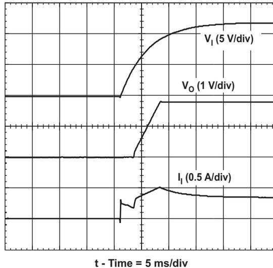
**Figure 11. Power-Up Waveforms**
