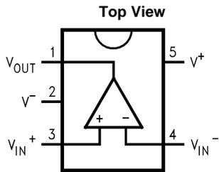
**Figure 34. 5-Pin SC70 and SOT-23 Packages
