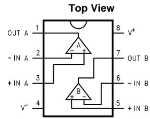
**Figure 35. 8-Pin SOIC and VSSOP Packages
