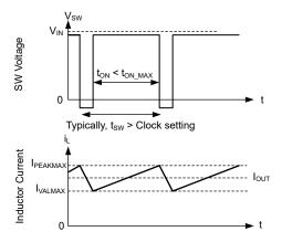
Figure 8-13. Current Limit Waveforms
