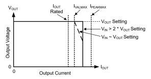
Figure 8-14. Output Voltage Versus Output Current
