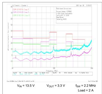
Figure 9-27. Typical CISPR 25 Radiated EMI 30 MHz–300 MHz Horizontal Bicon Antenna Blue: Peak Detect, Pink = Average Detect
