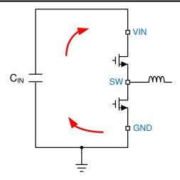
Figure 11-1. Current Loops with Fast Edges
