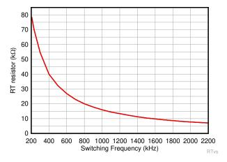
Figure 8-7. RT Values vs Frequency
