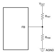
Figure 8-9. Setting Output Voltage for Adjustable Output Variant
