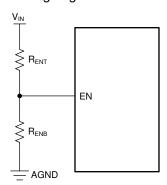
Figure 8-1. VIN UVLO Using the EN Pin
