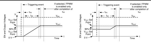
Figure 8-10. Soft Start With and Without Pre-bias Voltage
