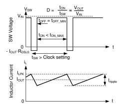
Switching waveforms while in dropout. Inductor current takes longer than a normal clock to reach the desired peak value. As a result, frequency drops. This frequency drop is limited by  $t_{\text{ON-MAX}}$ .
