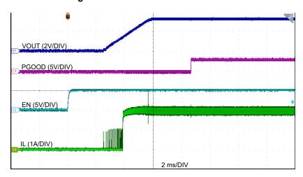
Figure 8-3. Enable Start-Up  $V_{IN}$  = 12 V,  $V_{OUT}$  = 3.3 V,  $I_{OUT}$  = 2 A
