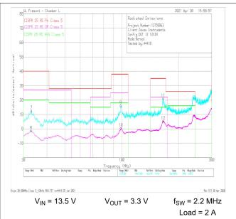
Figure 9-28. Typical CISPR 25 Radiated EMI 30 MHz–300 MHz Vertical Bicon Antenna Blue: Peak Detect, Pink = Average Detect
