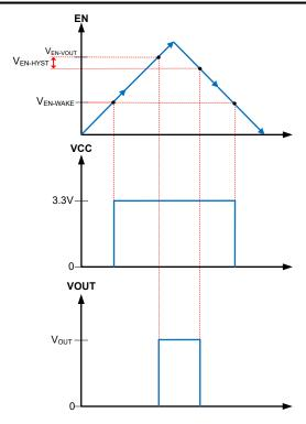
Figure 8-2. Precision Enable Behavior
