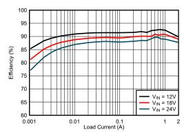
Efficiency:  $V_{OUT} = 3.3 \text{ V (Fixed)}$ , 2.2 MHz
