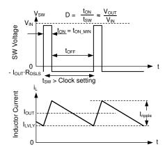
In valley control mode, minimum inductor current is regulated, not peak inductor current.
