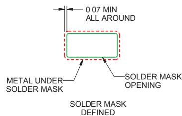
For recommended circuit layout for PCB designs, see [Reducing Ringing Through PCB Layout Techniques \(SLPA005\)](#).
