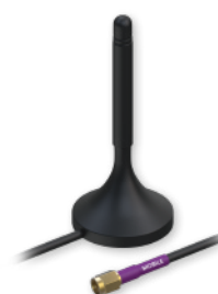
1 X BLUETOOTH ANTENNA (MAGNETIC MOUNT, RP-SMA MALE, 1.5 M CABLE)
