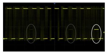
With a waveform update rate of up to 120,000 wfm/s, the oscilloscope can easily capture unusual or low-probability events. In Sequence mode, the waveform capture rate can reach 500,000 wfm/s.
