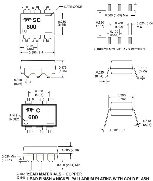
DIMENSIONS ARE SHOWN IN INCHES (MILLIMETERS) Tolerances (unless otherwise specified)
