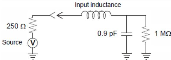
**Example Probe input equivalent circuit. Actual diagrams p.14.**
