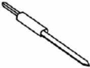
The Ground Blade and Copper Pad are intended to work together for the best grounding solution for probing an IC. The Ground Blade is designed to provide a short, low inductance ground path. The Copper Pad is adhesive backed to stick to the top of an IC, and can then be soldered to the IC ground.
