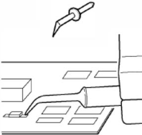
The Bent Tip is made out of titanium, this tip is ideal for situations that require the user to hold the probe parallel to the circuit board under test. Also gives you more control when holding the probe like a pencil. Fits in either probe socket. (PACC-PT005)
