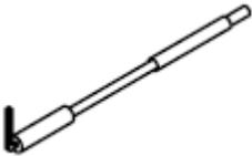
These leads have a socket on one end with a right angle and a square pin on the other to connect to the input or ground socket of the probe body, and may be used for general purpose probing.
