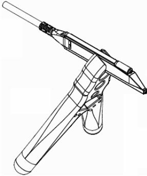
It is designed to keep most of the weight on the probe tip and will prevent lost contact when a bump to the table shakes the circuit under test.
