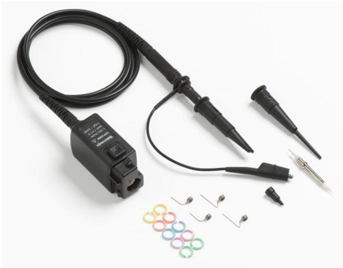
The TPP1000, TPP0500B, TPP0502 and TPP0250 models are high-bandwidth, general-purpose probes from Tektronix that offer breakthrough specifications previously unrealized in this product class. Designed for use with Tektronix MDO3000, MDO4000, MSO/DPO5000, and 5 Series MSO Series oscilloscopes, these probes provide up to 1 GHz of analog bandwidth with less than 3.9 pF of capacitive loading.
