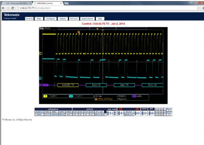
e\*Scope in a web browser showing the display of an MDO3000. Use e\*Scope to quickly document your work by saving screen images, waveforms, or setups for later use.
