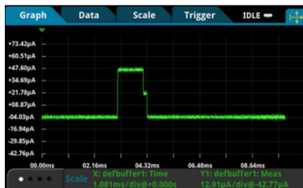
The high speed digitizing function allows capturing and displaying voltage and current waveforms.
