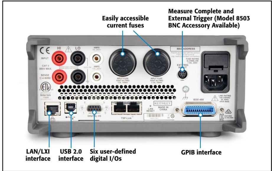
The rear panel of the DMM7510 provides connections and controls that simplify configuring multi-instrument test solutions, including input connectors, remote control interfaces (GPIB, USB 2.0, and LXI/Ethernet), a D-sub 9-pin digital I/O port (for internal/external trigger signals and handler control), and TSP-Link® jacks for connecting to other TSP-enabled instruments.
