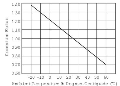
To use this chart: Read up from the ambient temperature to the curve, and across to find a correction factor. Multiply the breaker rating by the correction factor to determine the compensated rating. Calculate the overloads in terms of the compensated rating to use the published trip curve. Do not use these devices outside their specified operating temperature ranges.
