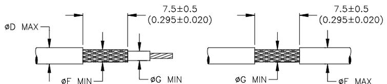
“G” is the minimum diameter on which the sleeve will seal.
