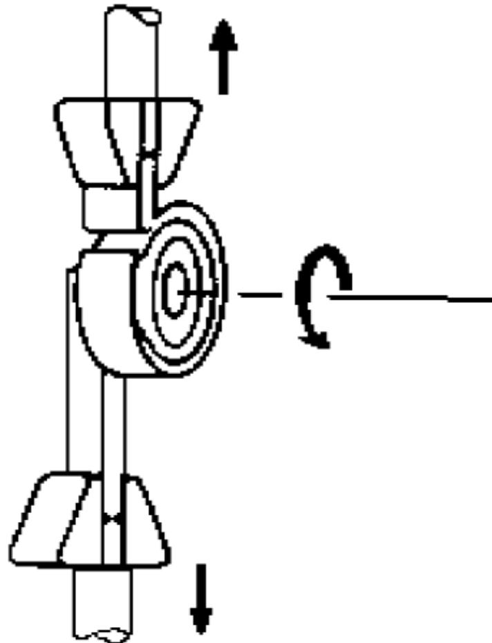
**FIGURE 1** Peel test specimen in Tensile Tester
