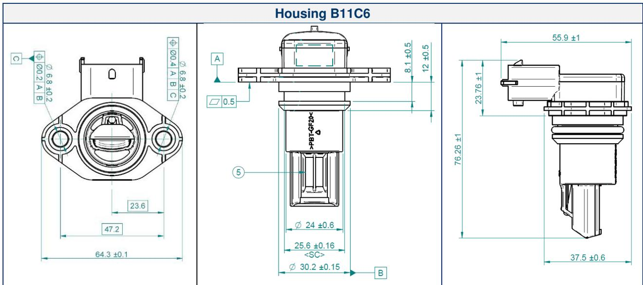
Recommended Screw Mounting: M6; Typical tightening torque: 12 N.m ; Maximum tightening torque: 17 N.m
