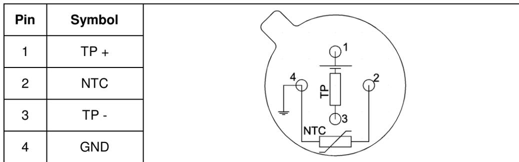
Figure 4: Electrical connections - bottom view of thermopile
