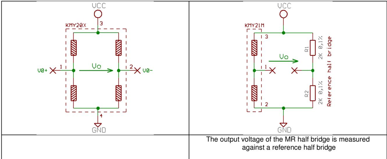
The output voltage of the MR half bridge is measured against a reference half bridge
