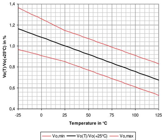
**Figure 6:** signal amplitude related to room temperature value
