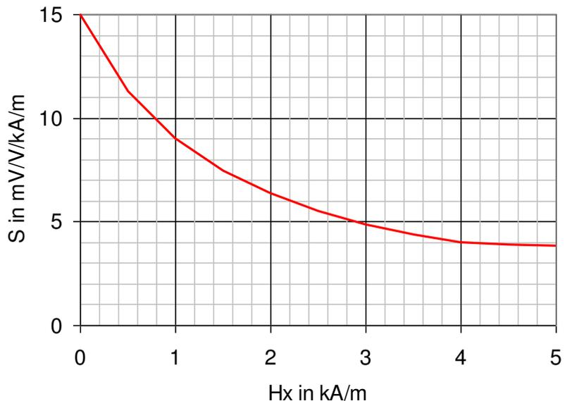
Auxiliary field strengths below  $H_x < 1.5$  kA/m are not recommended, as small disturbances may flip the magnetization domains. Sometimes, the magnetic conditions in the application may provide enough  $H_x$  bias field stabilization. MEAS Germany can provide advice for customer specific magnet arrangements.
