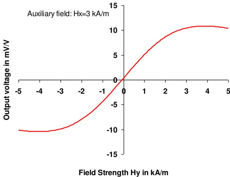
Figure 4: Characteristic output curve of KMY 20 S / KMY 22 / KMZ 20 S for an auxiliary field strength of  $H_x=3$  kA/m
