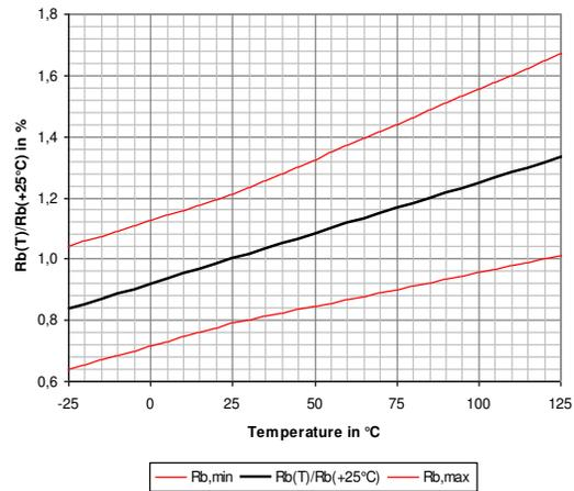
**Figure 7:** bridge resistance related to room temperature value
