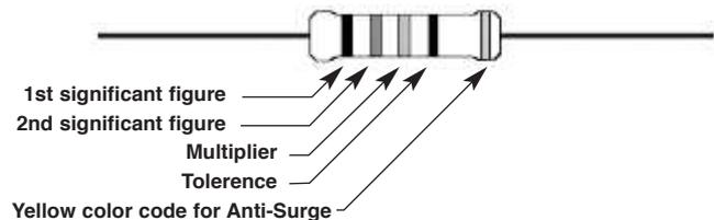
For EP Normal Size 5W, 7W, 8W 9W and EP Small Size 7WS, 8WS, 9WS, 10WS Resistors will be marked with power rating, nominal resistance and resistance tolerance code.
