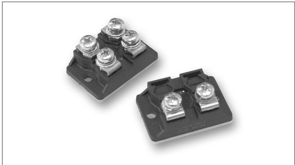
With less than 40nH inductance and a 100Watt power rating in an easy-mounting 38mm x 25mm Isotop case, the BDS100 offers high power density over a wide range of ohmic values (R47 – 1MΩ) and benefits from 10 years experience in the field. Available in 6 resistor configurations with 2 or 4 easy to connect terminals, the resistors are made from quality materials for optimum reliability and stability with very low partial discharge.
