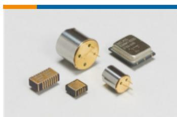
Embedded Accelerometers (15)
