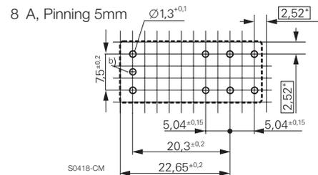
\*) With the recommended PCB hole sizes a grid pattern from 2.5mm to 2.54mm can be used.
