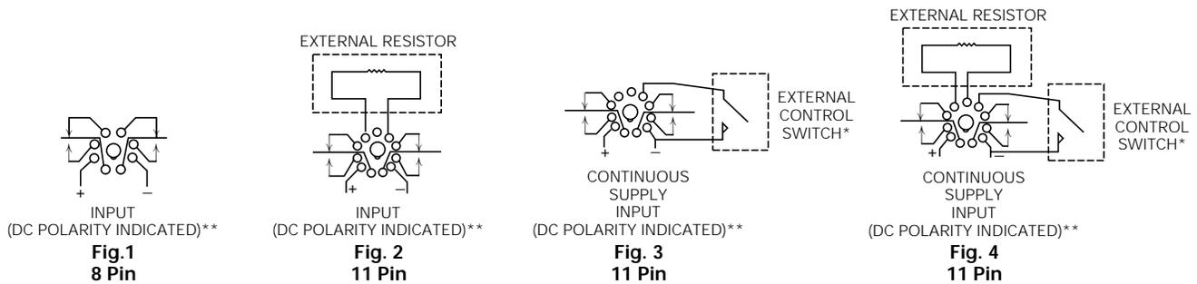
\* If control switch is closed when power is applied, relay will immediately energize. A 50 millisecond minimum switch closure is required. IMPORTANT: A dry circuit switch is recommended. A \* dry circuit\* switch is one rated to reliably switch currents of less than 50mA. Use of a switch rated for other than dry circuit may result in failure of the time delay relay to function properly.
