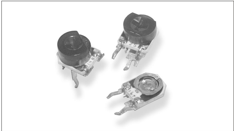
This tiny 6mm square cermet trimmer is offered with alternative adjustment covers for screwdriver and automatic setting and can be supplied in bulk or taped in ammo pack. The 416 can be adjusted from the top or side and is an inexpensive solution to high reliability potentiometer requirements. This series is used to replace some of the larger, expensive, sealed types in high volume circuits.
