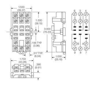
Screw terminal, DIN rail, snap-mount socket 27E893 Offers screw termination for KUEP, KUGP, KUIP, KUL, KUMP and KUP relays, through 3 poles, with .187" (4.75mm) quick connect terminals. Also used with CL/CU time delay relays. This socket is constructed with a spring-loaded latch which allows it to be quickly snapped onto or removed from a DIN or "top hat" style mounting track. No special tools or extra hardware is required for installation
