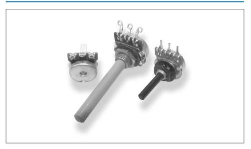
A popular range of 20mm control potentiometers, the type 23 series can be tailored to suit more specific requirements. The potentiometers are available with printed carbon resistance element, choice of bush lengths in metal or plastic and insulated shafts up to 50mm in length. In addition, approved mains and low current switches are available as standard options.
