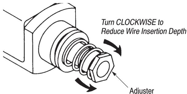
Turn **COUNTERCLOCKWISE** to Increase Wire Insertion Depth
