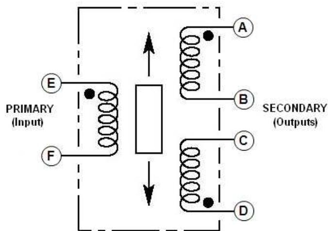
A through F: Connector pin assignments
