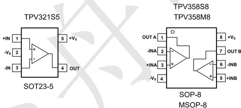
**FPin Assignment Diagram (SOT23-5 and SOP-8 MSOP-8 Package)**
