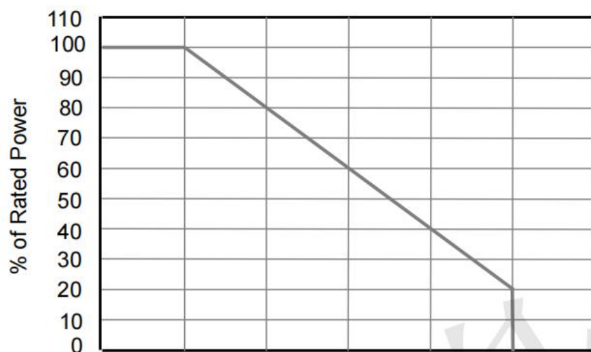
Fig3. Power Derating Curve
