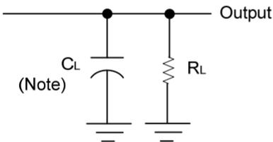
Note:  $C_L$  includes probe and jig capacitance.
